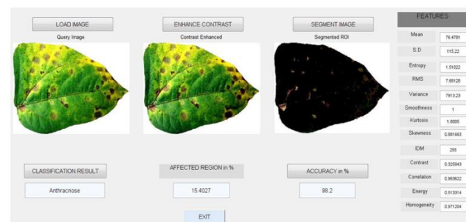
System shows leaf disease detection of P. vulgaris using digital image processing techniques
